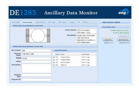
The upper portion of the screen contains the AFD Decoder module which displays the current AFD code on the top right of the module, the de-coded aspect ratio description below the code, and a visual representa-tion of the AFD code on the left hand side. The default viewing option shows the AFD Decoder display. To hide the AFD decoder module, click on the upwards arrow at the top right hand corner. To expand the mod-ule, click the downwards arrow at the top right hand corner.
