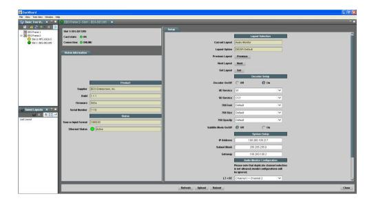
There are two main sections in the DashBoard interface: the Status in-formation on the left side and the Setup menu on the right side. At the bottom of the DashBoard there are four general purpose buttons. The **Refresh** button updates the fields on the DashBoard to reflect the card's current state. The **Upload** button prompts the user to select an upgrade file to apply to the card. The **Reboot** button restarts the card itself. The **Close** button closes the frame card interface.
